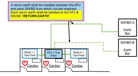
Three separate cardiac areas with one EP earthing system comprising the EP junction and node facility.
