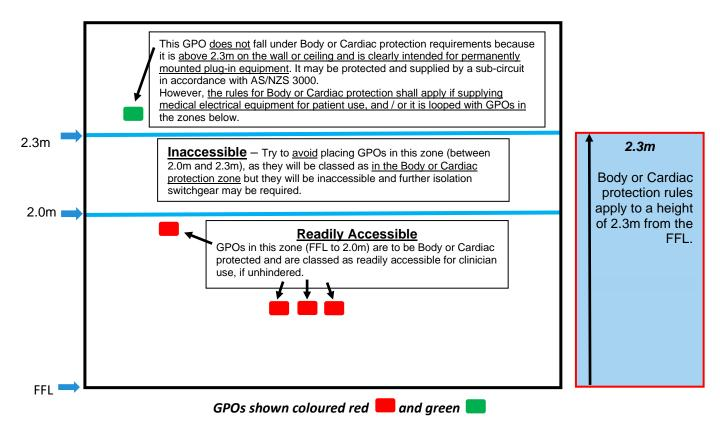
This electrical standard is quite specific in that the body-protected or cardiac-protected electrical areas medical electrical equipment *must be in the control of the clinician within the area*:
