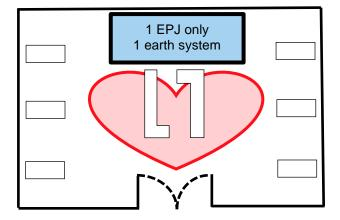
**CL.4.4.2.3** – (cardiac bonding) A EP earthing system may have a number of separate nodes at strategic locations connected to the EP junction.
