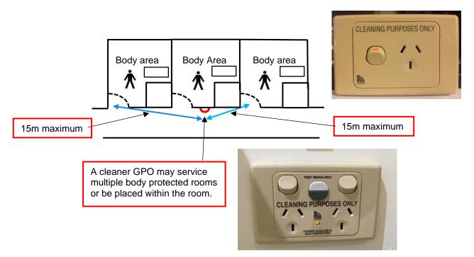
**CL.1.5.12** – (socket-outlets) Groups of socket-outlets must have clear delineation (e.g. stainless steel medical panel with a combination of different GPO supplies, an engraved line between GPO services or clear separation for easy user understanding).
