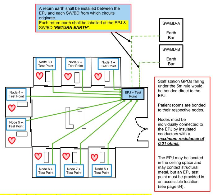
**CL.4.4.2.3 (b)** – (cardiac bonding) Each node is accessible and its location identified by labelling.
